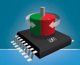
**AS5311** First magnetic encoder to break into submicron resolution range
